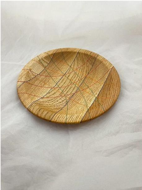
The bowl is made from American White Oak salvaged from bags of firewood. Having first planed them up by hand they were then joined with stained veneer in between. It was then cut up into three pieces and re-joined with more coloured veneers, this process was then done twice more before cutting to round and turning and finished with four coats of oil. [DR]
