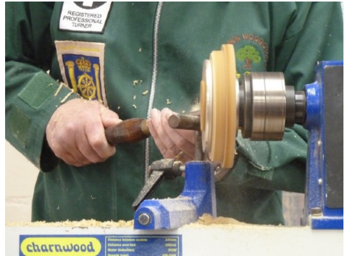
The pewter rim was released from the MDF mould.
